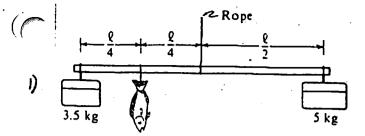
To weigh a fish, a person hangs a tackle box of mass 3.5 kilograms and a cooler of mass 5 kilograms from the ends of a uniform rigid pole that is suspended by a rope attached to its center. The system halances when the fish hangs at a point  $\frac{1}{4}$  of the rod's length from the tackle box. What is the mass of the fish?
