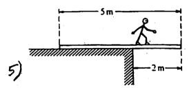
A 5-meter uniform plank of mass 100 kilograms rests on the top of a building with 2 meters extended over the edge as shown above. How far can a 50-kilogram person venture past the edge of the building on the plank before the plank just begins to tip?
